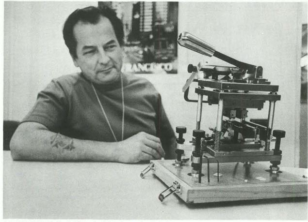
A MOON LANDER it's not. It's a lead forming and cutting device invented by Don Dubose, and it's capable of forming the leads on most of the common flat packs.
